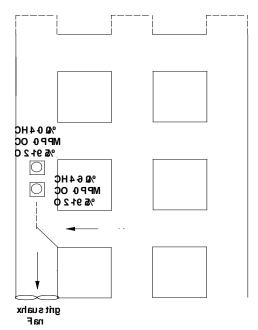
Rule 48 defines an exception that allows one circumstance where ventilation structures may be placed other than perpendicular across and entry, crosscut, or opening. The exception is "Brattice frames and brattice cloth, may be used to erect a line curtain which can only extend from a face, barricade, or airtight separation to the outby intersection."
