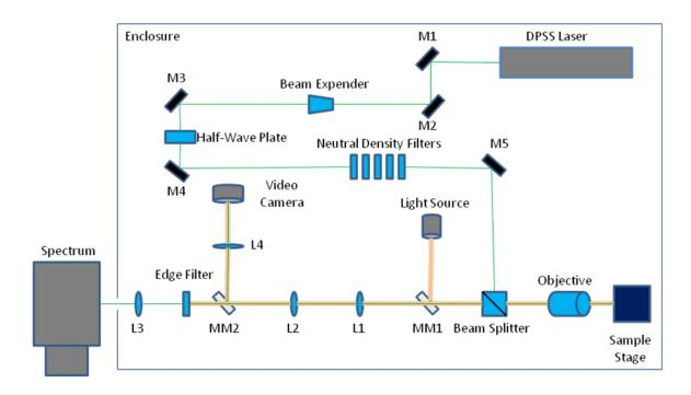
M: reflecting mirror; MM: movable mirror; L: focus lens
