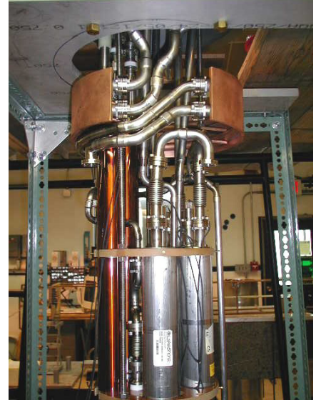
Figure 2. Vertical Test Facility for magnetic measurements of future superconducting undulators.
