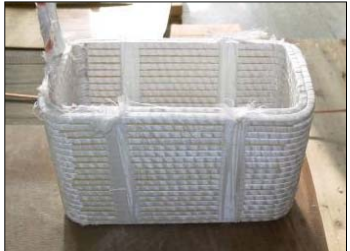
Figure 1: Quadrupole coil ready for vacuum impregnation at BINP.
