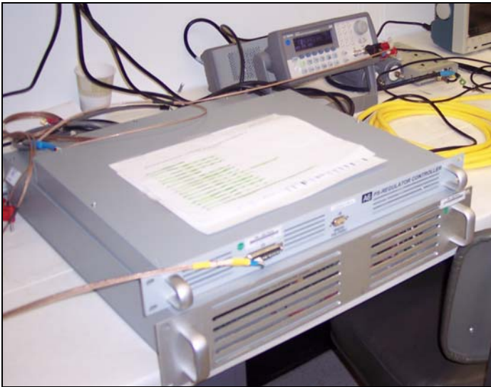
Figure 2: Test setup of Fast Corrector Power Supply.
