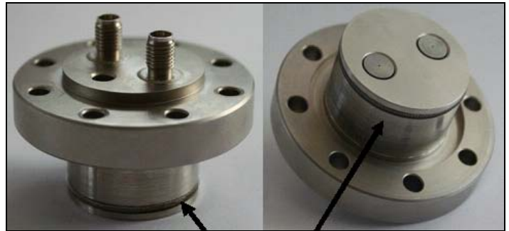
Figure 3. Production RF BPM button assembly with groove for RF spring ring to suppress longitudinal impedance mode.
