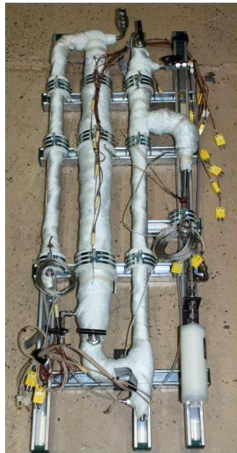
FIGURE 4. 2-Stage Dilution Tunnel Constructed at ORNL to Measure Particle Emissions with the Scanning Mobility Particle Sizer Instrument
