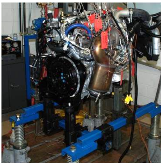
FIGURE 1. 4-Cylinder Research Engine for Ethanol Optimization Modified from a Production Engine by ORNL's CRADA Partner Delphi
