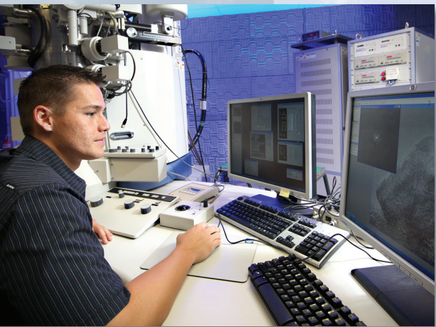
Transmission electron microscopy for in situ characterization studies helps evaluate the stability of battery electrode materials during rapid charge-discharge cycling.
