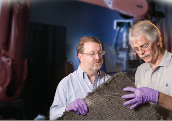
Researchers examine a carbon-fiber composite preform. Such a lightweight material could improve a car's fuel economy.
