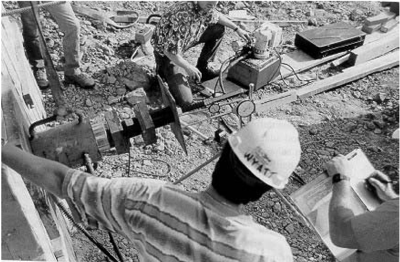
Figure 8.1: Soil Nail Load Testing Setup.
