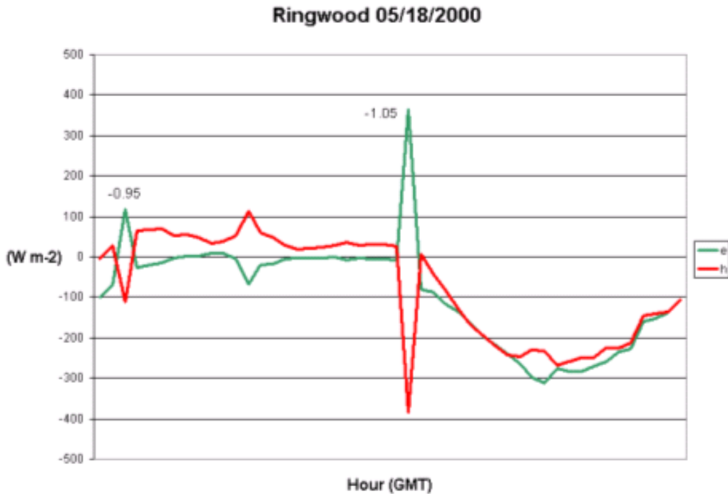
Figure 1. Plot showing sensible (h) and latent (e) heat fluxes showing a normal diurnal variation in heat fluxes. Spikes in the data occur at sunrise and sunset when the Bowen ratio is near -1.
