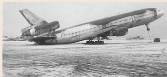
The weight of rain-soaked ash fall from the 1991 eruption at Pinatubo Volcano in the Philippines caused this DC-10 to fall back on its tail at Cubi Point Naval Air Station (photo courtesy of R.L. Rieger/U.S. Navy). An inch of wet ash can weigh as much as 10 pounds per square foot.
