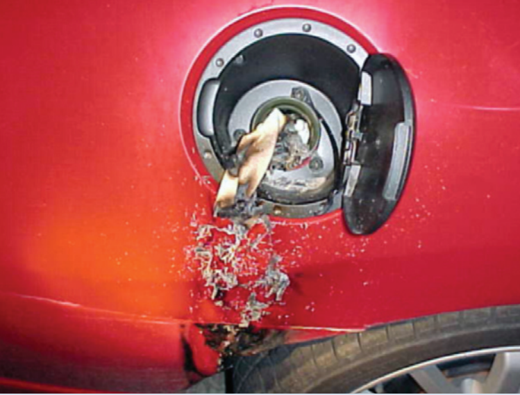
Deliberate fire set at the opening of a gas tank.
