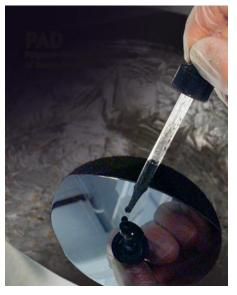
LANL's solar power portfolio includes a deposition process known as PAD. PAD eliminates the need for vacuum-based thin film equipment. In the photo, a researcher applies a PAD solution to a silicon wafer prior to spin coating.
