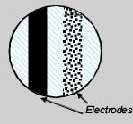
O Spray on a thin film of electrolyte over part of the sensor
