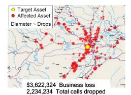
This graphic depicts a virtual telecommunications grid. The yellow dot represents a central communications switch. The red dots represent each outlying user associated with that switch. LANL, through the use of MIITS, predicts that the failure of the hub will result in the cumulative telecommunications loss of each outlying user.
