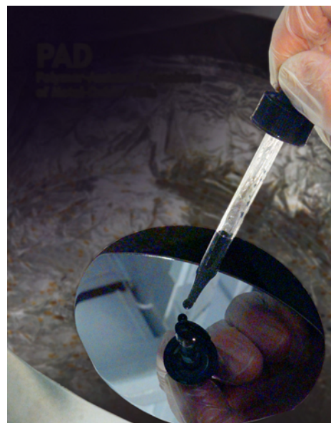
A researcher applies a few drops of a water-based PAD solution to a silicon wafer mounted on a spin-coater.
