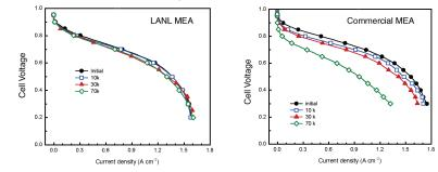
Polarization curves after cycling test of premier manufacturer's MEA and LANL's MEA. Curves were obtained at 0k, 10k, 30k, and 70k of potential cycles from 0.6 to 1.0 V in H<sub>2</sub>/N<sub>2</sub> conditions. The pt loading was 0.2 and 0.4 mg/cm<sup>2</sup> for both the LANL and premier manufacturer MEAs respectively.
