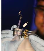
very inexpensive, rectangular cuvettes instead of custom cells. Experimental setups can use holes in the caps for insertion of a reference electrode, a counter electrode, or as a gas inlet and outlet. Optional holes in the bottom and sides of the cuvettes can be used for electrical connections, tubing, or filtration. The same cell can be used for bulk electrolysis and surface electrochemical experiments.
