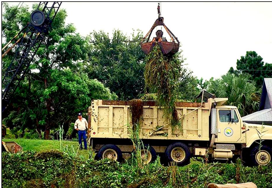
Figure A-13. Equipment can become contaminated with pest and invasive species during field work. Contaminated equipment can spread these species to uninfested sites. Inspect and clean equipment before moving to a new work location.
