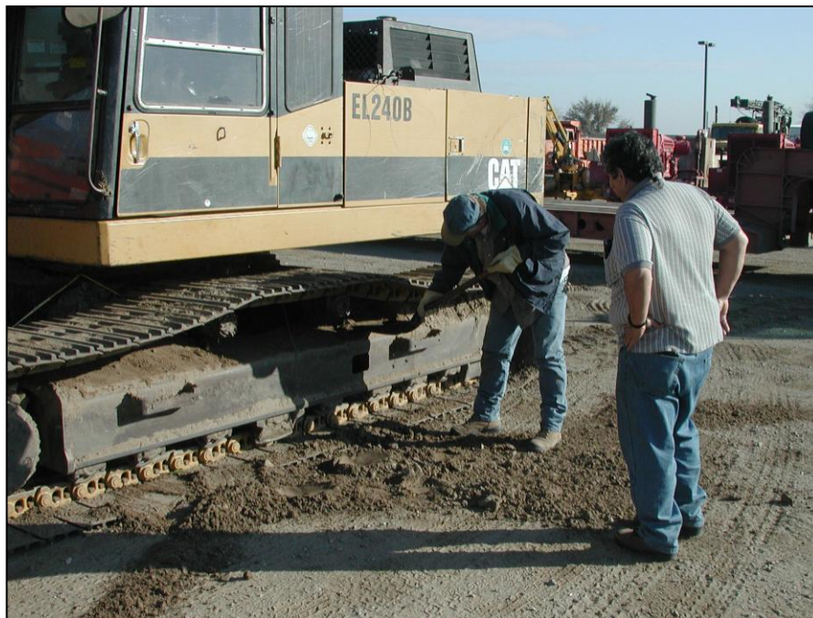
Figure 7. Precleaning heavy accumulations can help reduce water use when washing. Working in certain areas may require a safety lookout (photo courtesy of Fred Nibling).
