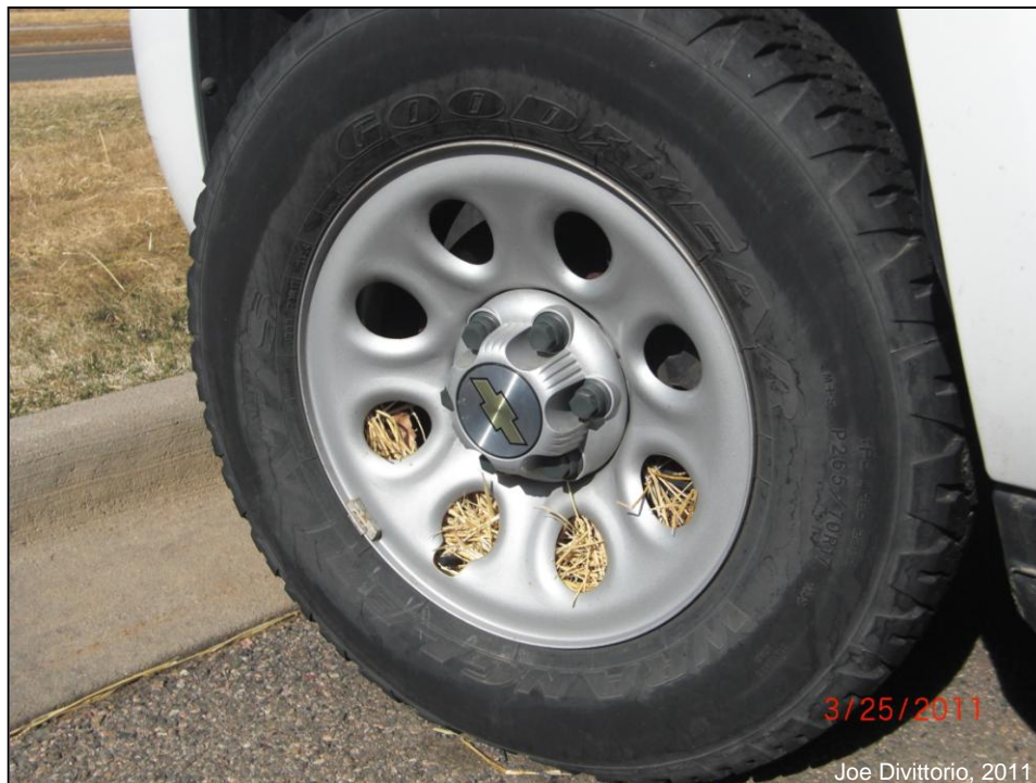
Figure A-14. A packrat nest constructed around the disk brake inside the front wheel of a vehicle. The major nest building material is straw, which was being used as a soil erosion control treatment at a nearby construction site (photo courtesy of Joe DiVittorio, 2011).
