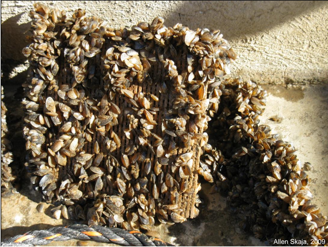
Figure B-12. This 90-10 copper nickel fish screen has been exposed for 4 months; notice the amount of mussels attached to the surface (photo courtesy of Allen Skaja, 2009).
