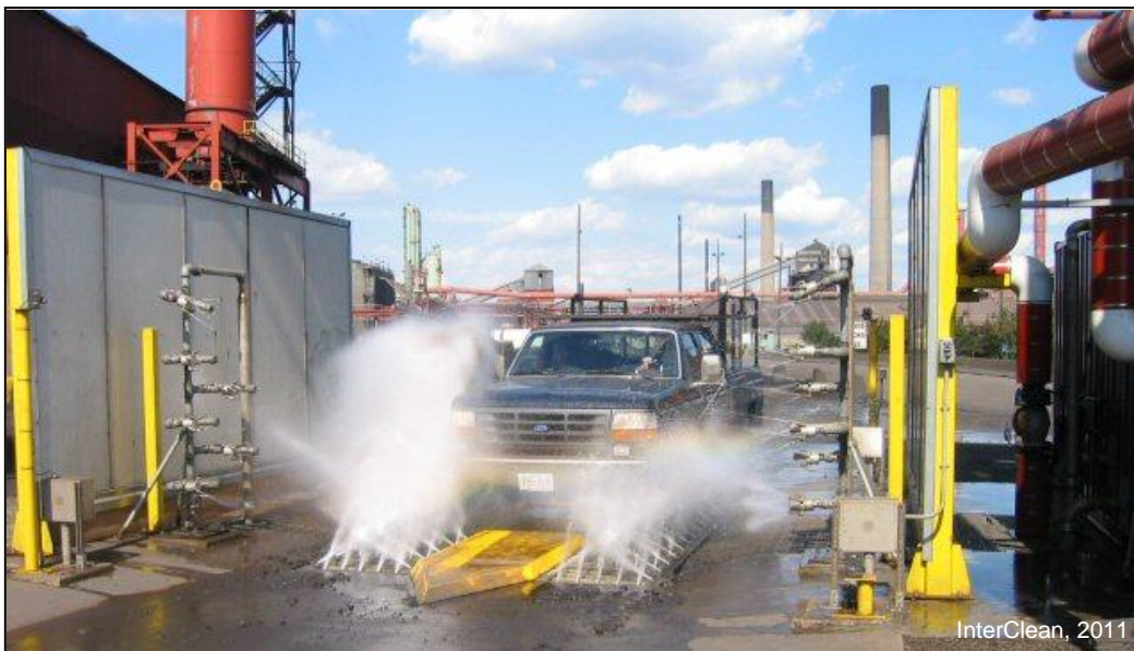
Figure B-5. InterClean Equipment's heavy duty washing system (InterClean, 2011).
