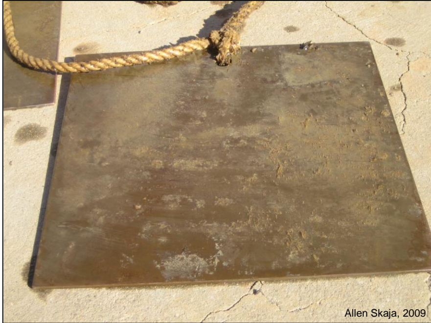
Figure B-10. This brass plate has been submerged for 18 months in Lake Havasu; notice there are no mussels on the rope or on the plate (photo courtesy of Allen Skaja, 2009).
