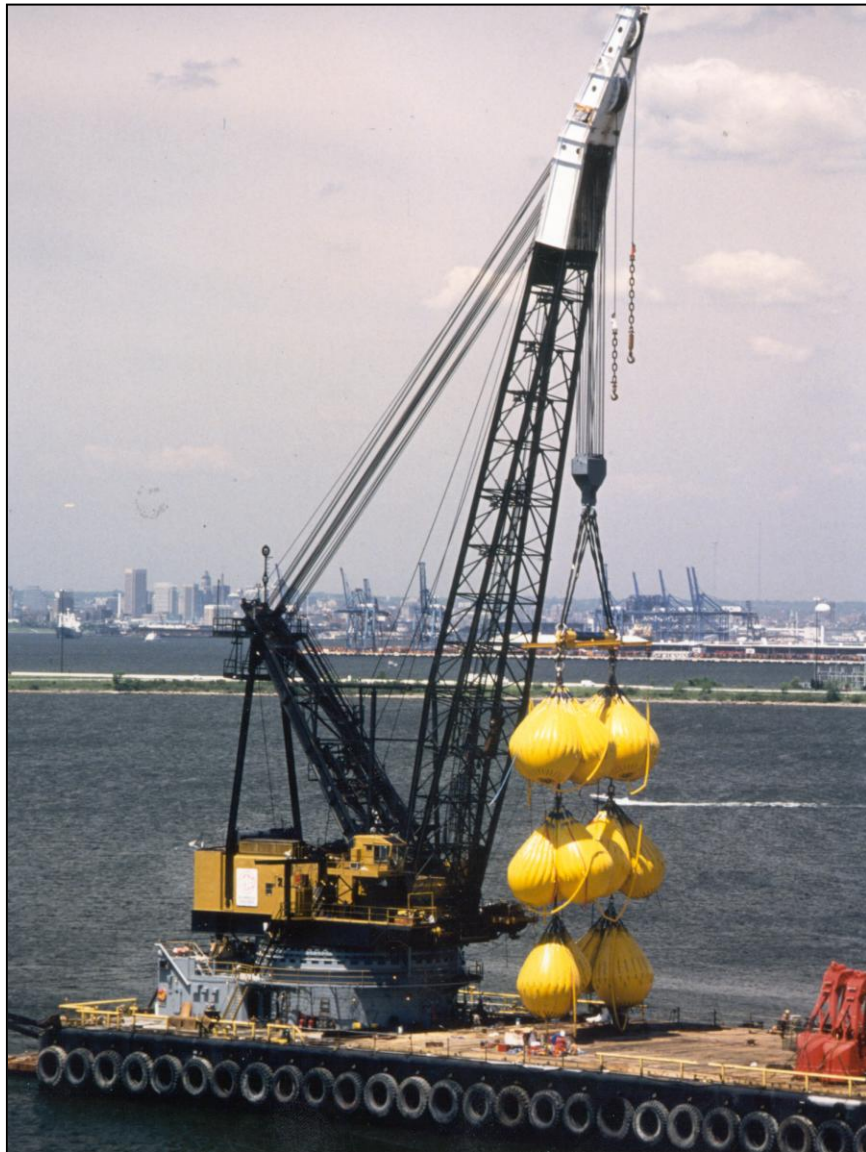
Figure A-12. The 'Betty L' Barge Crane, Morrison Knudsen Company, during water weight bag™ testing, Baltimore, Maryland (photo courtesy of Jim Jota, Imes, Inc., 1994).
