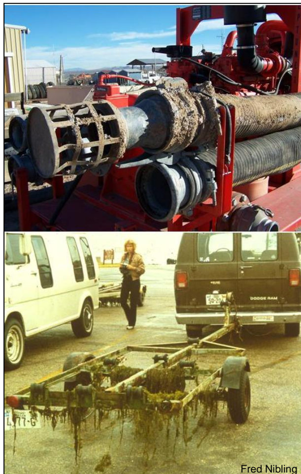
Figure 13. Mud and debris on pump (above) and hydrilla on boat trailer (below) (photo courtesy of Fred Nibling).
