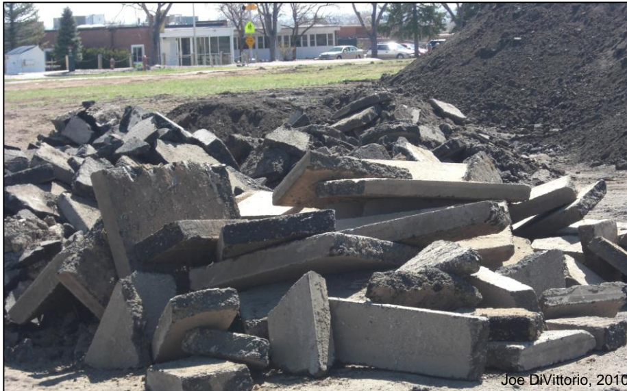
Figure A-3. Stockpiled broken concrete – note contact surfaces with adhering residue soils. These surfaces can harbor foreign species from the site of previous use (photo courtesy of Joe DiVittorio, 2010).
