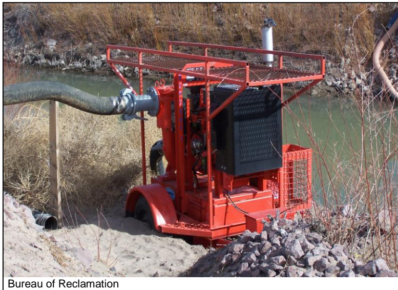
Figure B-3. Water for vehicle cleaning was pumped from conveyance channel at Socorro, New Mexico field site (Bureau of Reclamation photo).
