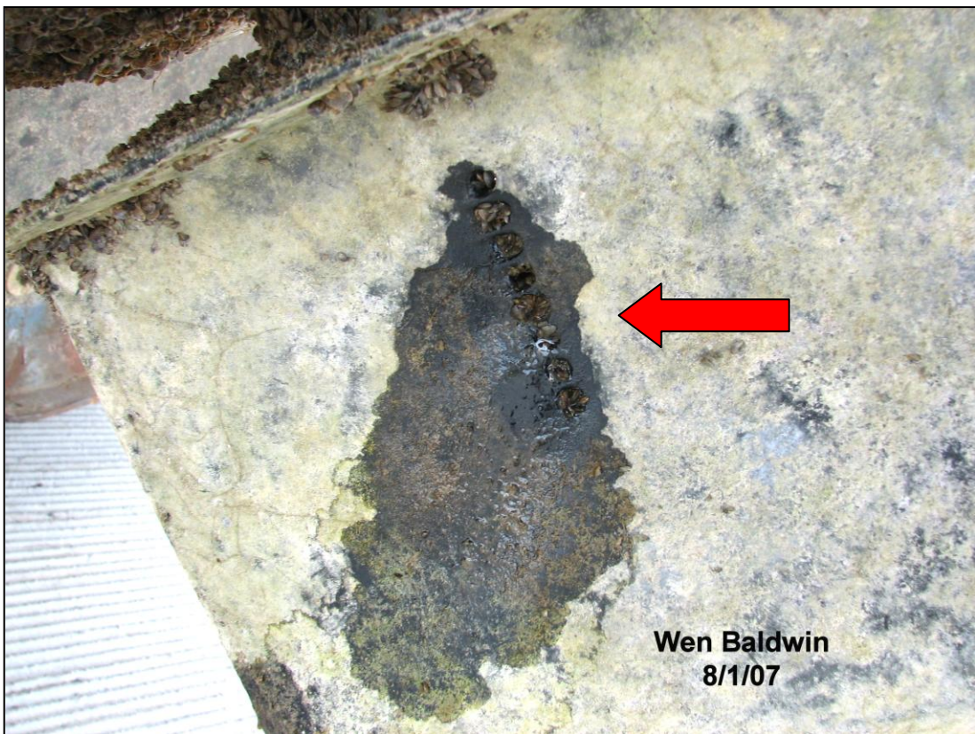
Figure A-8. Closeup view of outboard motor shaft housing. Adult quagga mussels living inside the engine and plugging the water intake ports of this outboard motor.
