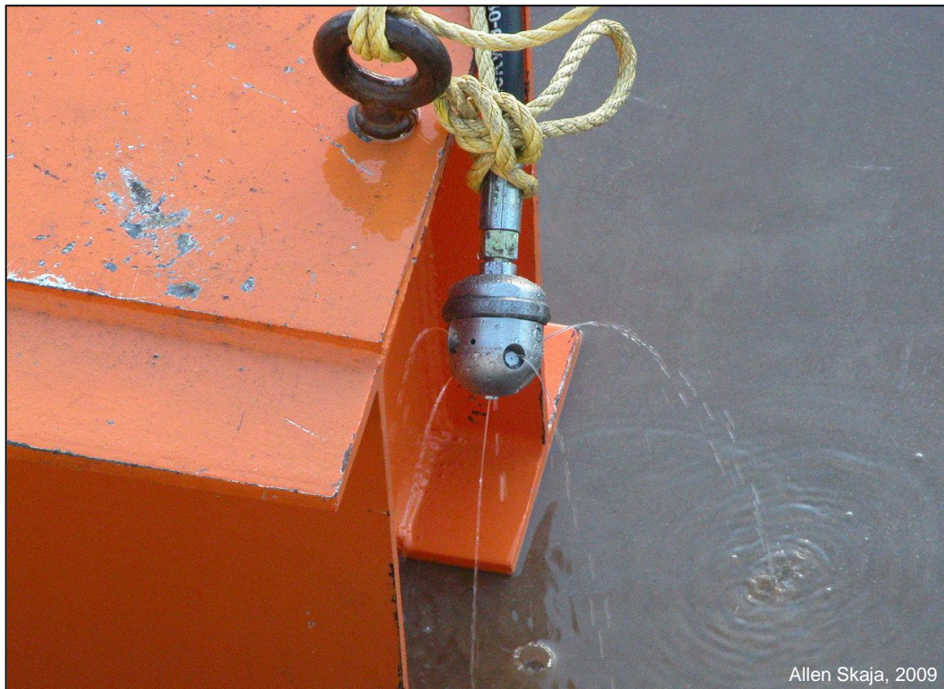
Figure B-8. Water jetting spin nozzle for cleaning out small diameter pipe infested with quagga mussels (photo courtesy of Allen Skaja, 2009).
