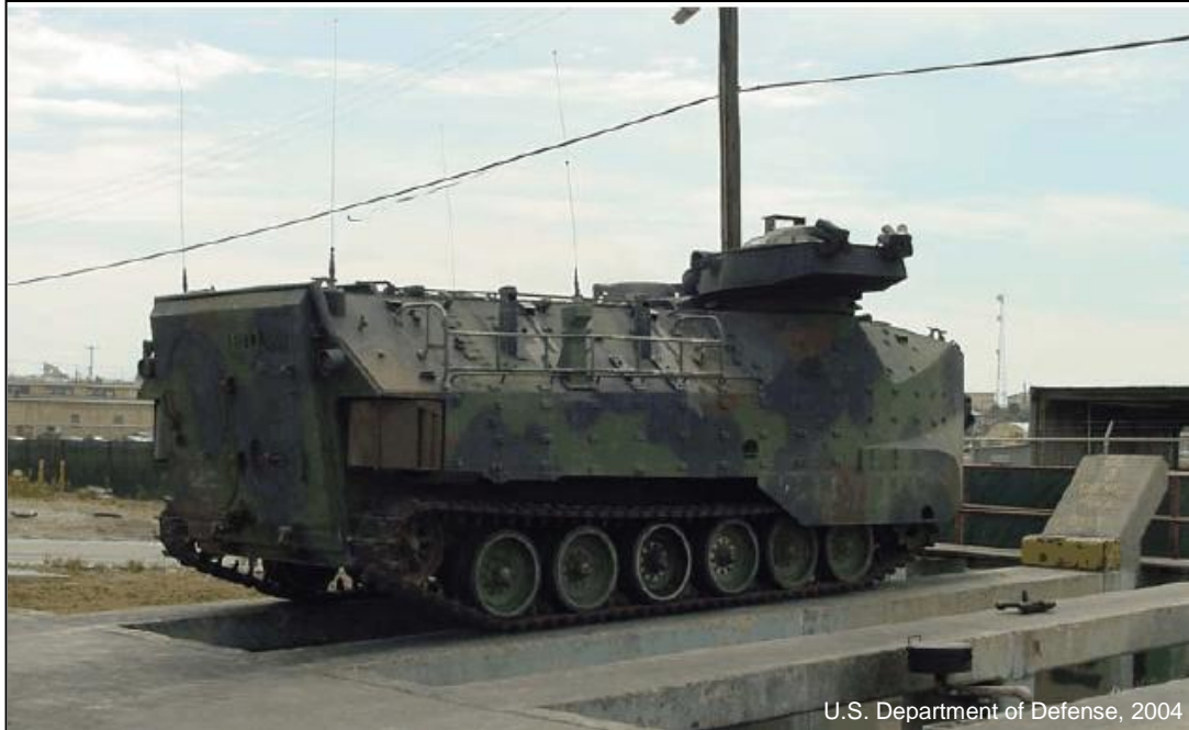
Figure 15. Tracked military equipment wash bay with hardstand surface and access underneath equipment (U.S. Department of Defense photo, 2004).
