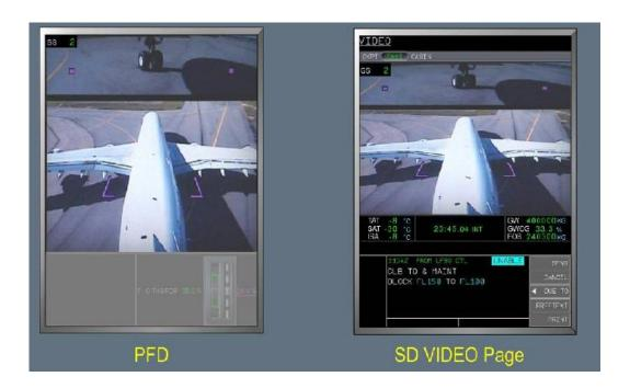
Figure. Live camera views on an A380 as shown on the PFD and SD.
