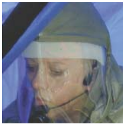
“Temple-transducer” style two-way radio headset stays in place under PAPER hoods.
