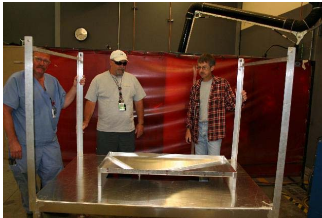
Completed drain pan assembly for WRPS Tank Field Operations.
