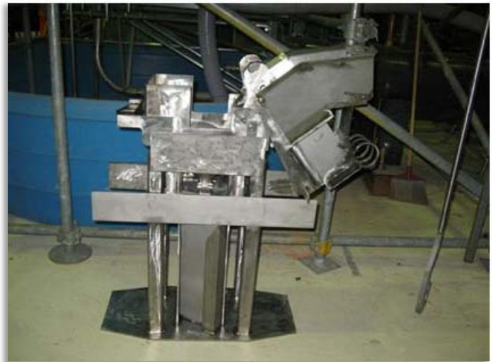
Knockout Pot Insert Loading Test Setup
