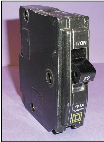
Figure 8: A Counterfeit Square D Circuit Breaker
