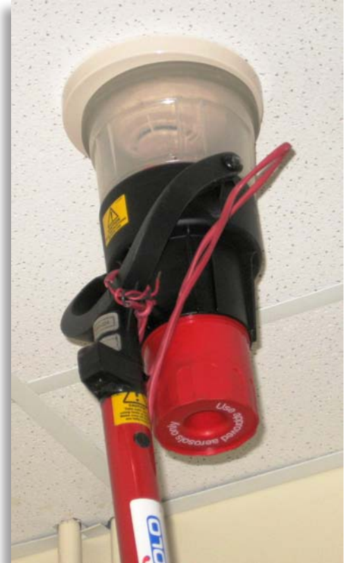
This device is used to test detector performance. Other equipment is used to test sensitivity.
