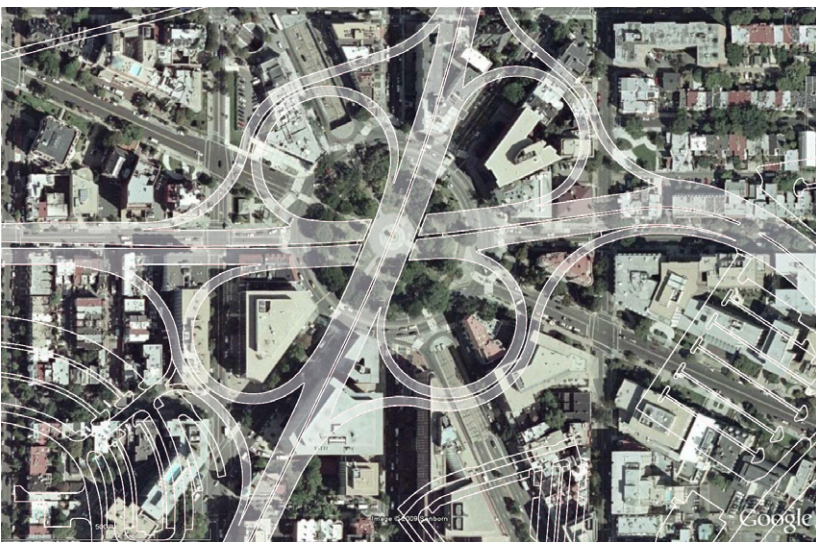
Scale Overlay of Cloverleaf on Dupont Circle - Traffic can be handled in a more compact and pedestrian-friendly environment that offers opportunities for community open space and beneficial development
