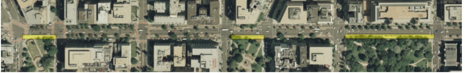
Figure 20 – Proposed K Street corridor, with a consistent corridor width. Areas that need to be widened are highlighted in yellow.
