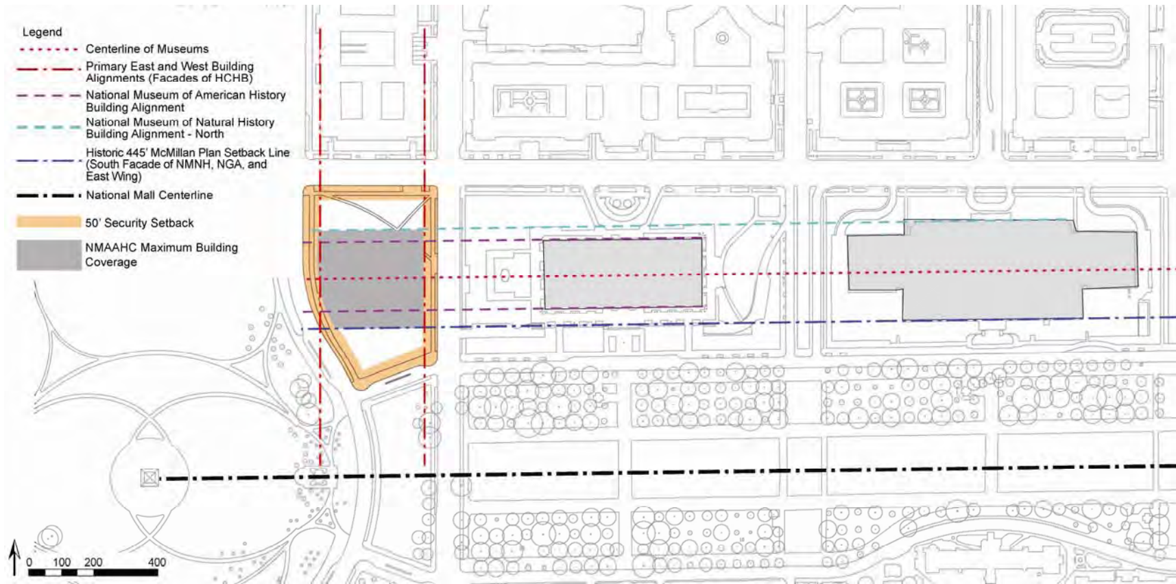
Figure 2.1.1 Tier II Setback and Building Alignment Lines
