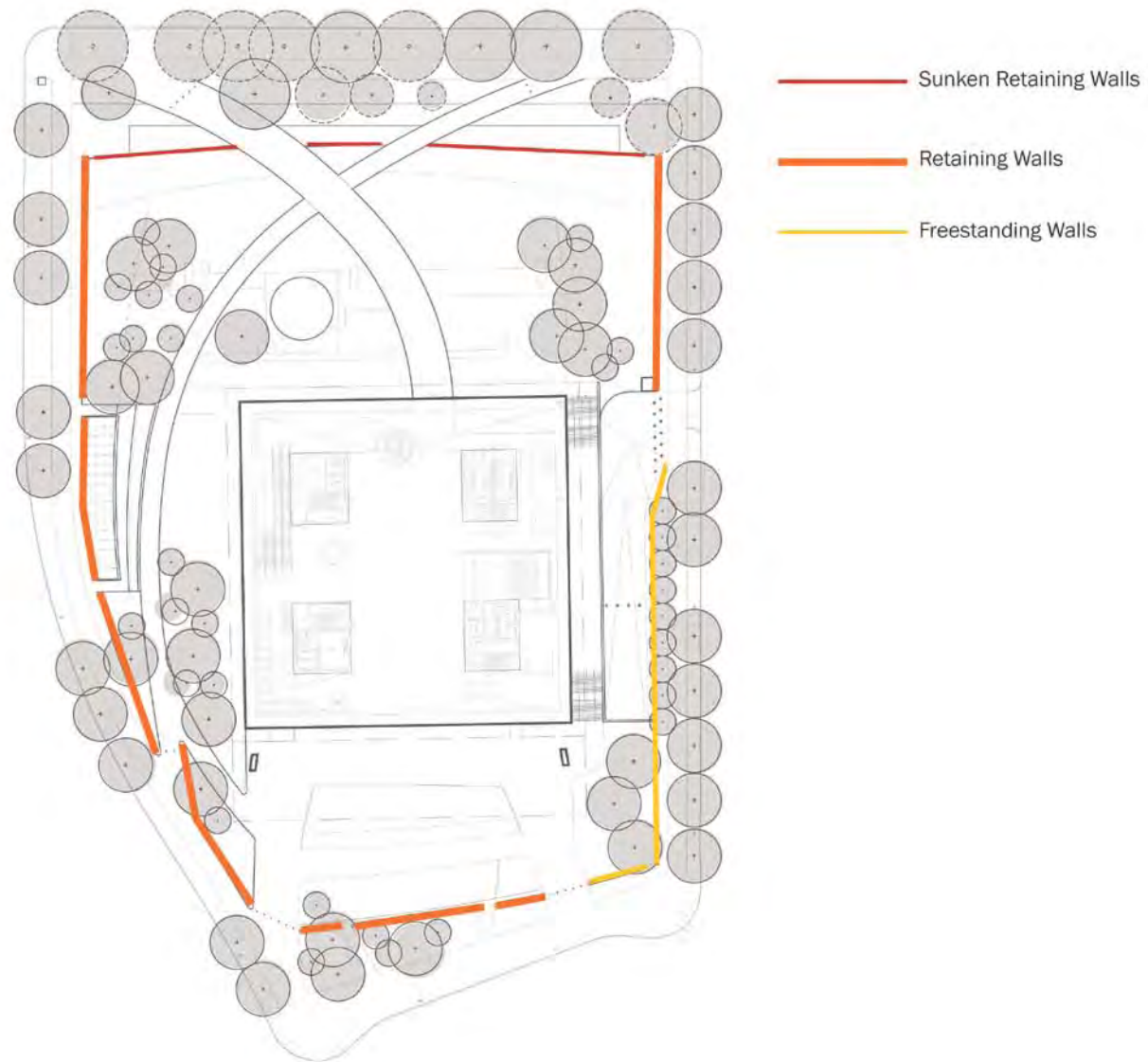
Figure B.1.7 Perimeter Security for the Refined Pavilion 2 - Preferred Alternative Source: Gustafson Guthrie Nichol, 2011
