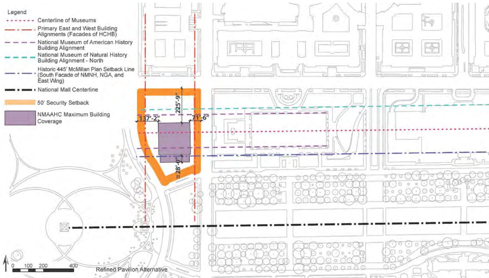
Figure 3.4.9 Refined Pavilion Alternative: Building Alignment
