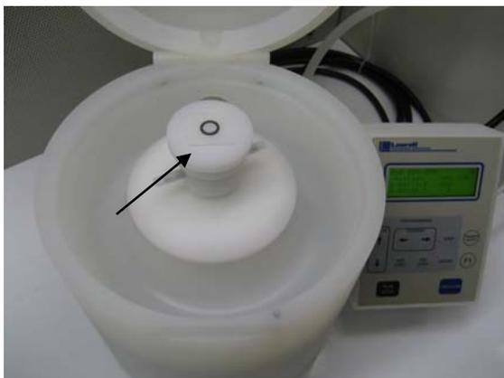
**Figure 14. Image of the Spin Coater Used with the Glass Substrate in Place on the Chuck**
