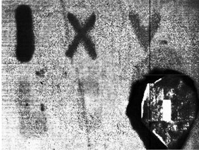
Figure 4. Image of a polyester fabric with lettering made from blood. The letter “I” was made with neat blood, while the letters “X”, “V”, “L” and “C” were made using blood of 10-, 25-, 50- and 100-fold dilutions. This image was made using in-phase detection of an AC-modulated reflectance. The object in the lower right is a reflectance reference for phase detection. 36
