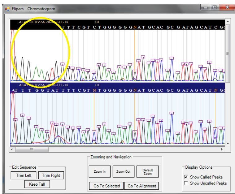
Figure 7: An (unrealistic) example of how trimming in the chromatogram works. Trim left was used to remove all base calls to the left of a particular position - the invalidated peak calls are circled in yellow.
