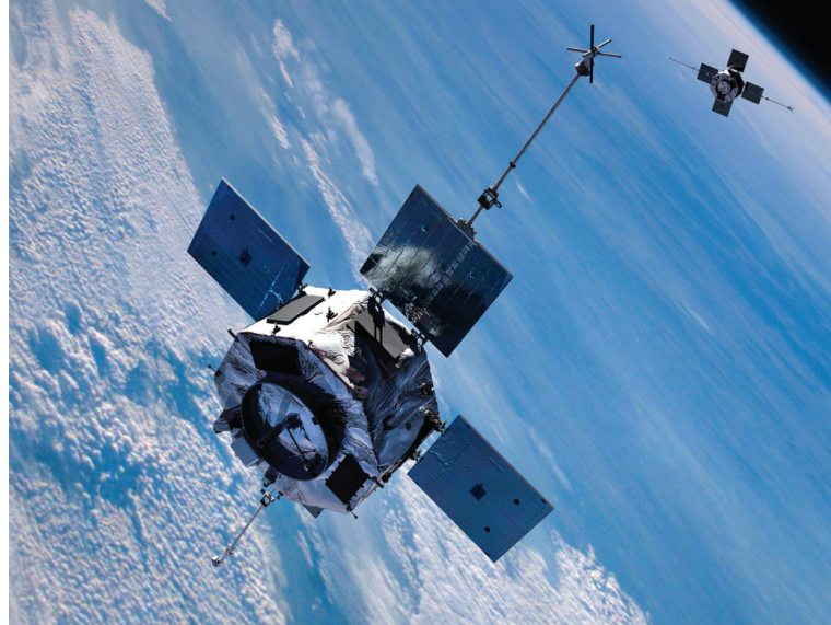
The Radiation Belt Storm Probes, a matched pair of satellites designed to gather the data needed to understand the dynamics of the radiation belts, are scheduled to be launched in the fall of 2012. Los Alamos was heavily involved in justifying and defining their mission and in designing a suite of instruments carried on each probe, including building one of the instruments (the HOPE spectrometer). This is an artist's rendering of the probes in orbit.
