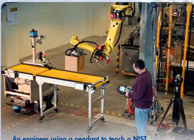
An engineer using a pendant to teach a NIST robot how to handle packages delivered to a conveyor by an automated guided vehicle.
