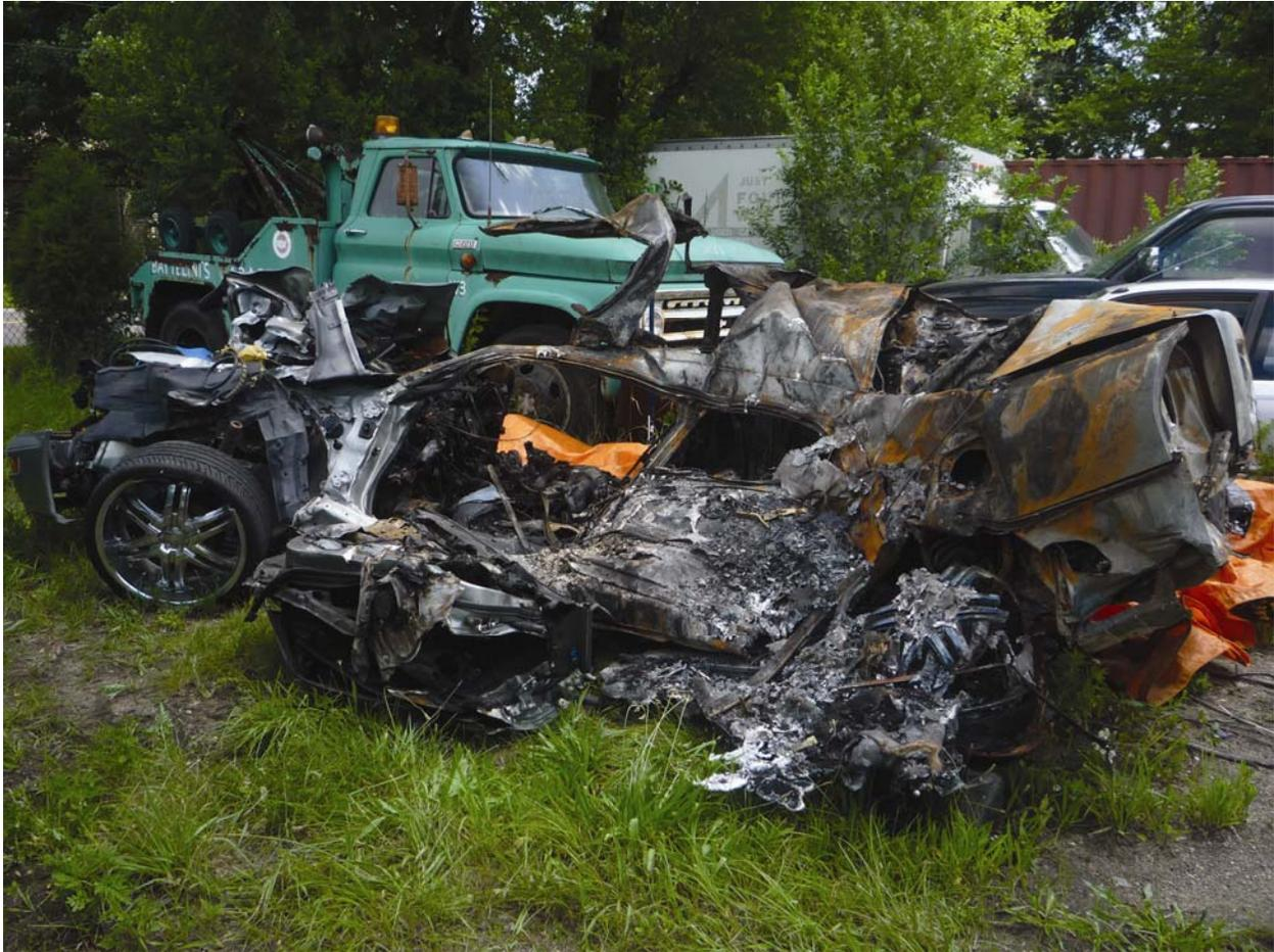
**Figure 3.** Left side view of automobile showing damage from collision and fire.
