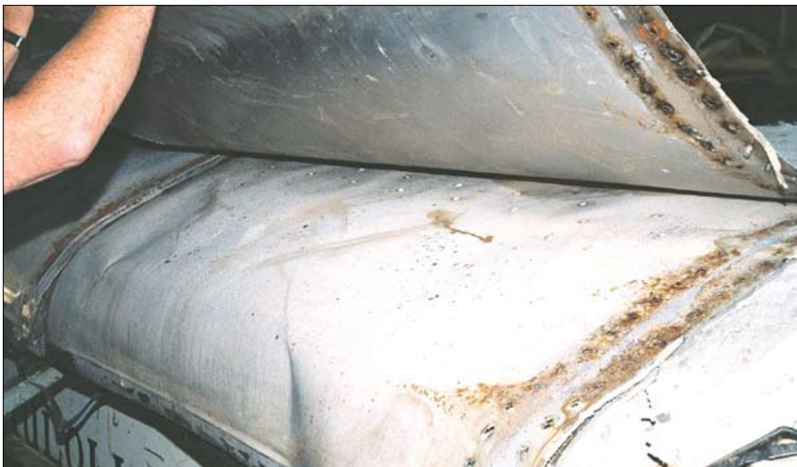
Figure 3. Roof of motorcoach, postaccident.
