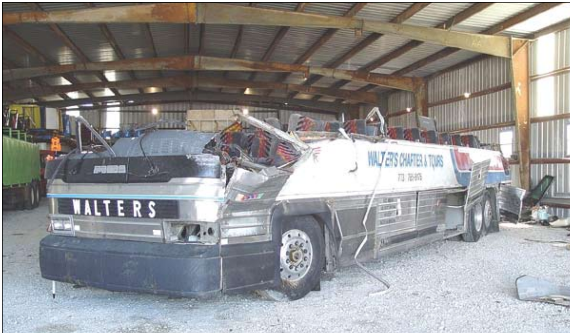
Figure 2. Motorcoach postaccident, with roof detached.
