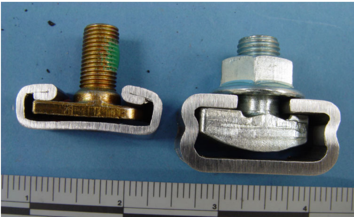
Figure 12. Exemplar T-bolt and floor track hardware for Neoplan (left) and National Seating (right).
