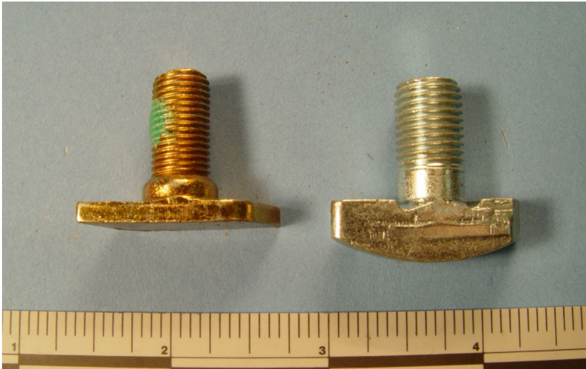
Figure 13. Exemplar T-bolt top section and length measurement for Neoplan (left) and National Seating (right).
