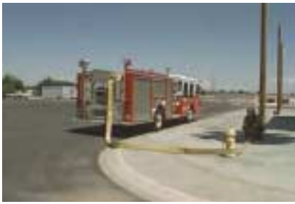
(Fig. 2.16a) Pumper stopping to initiate a forward hose lay from a hydrant.
