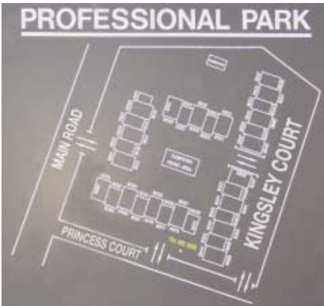
(Fig. 2.13) Diagrammatic sign showing an entire complex of buildings and their address(es). The addition of fire hydrant locations (and any other fire protection features) would assist responding firefighters.
