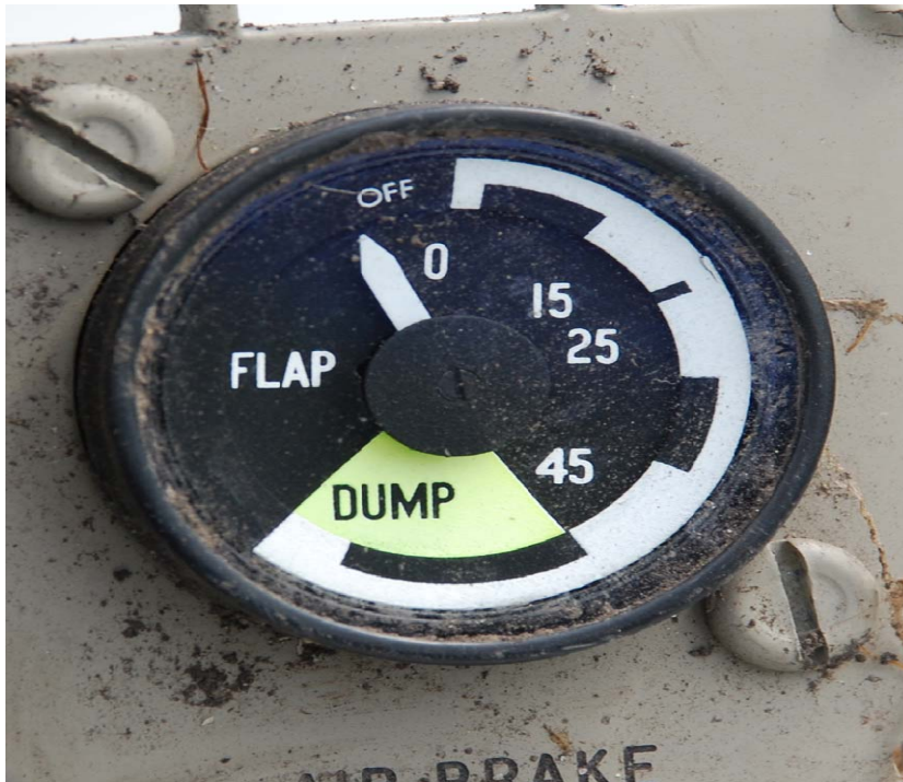
Figure 2. Photograph showing the accident airplane's mechanical flaps indicator.
