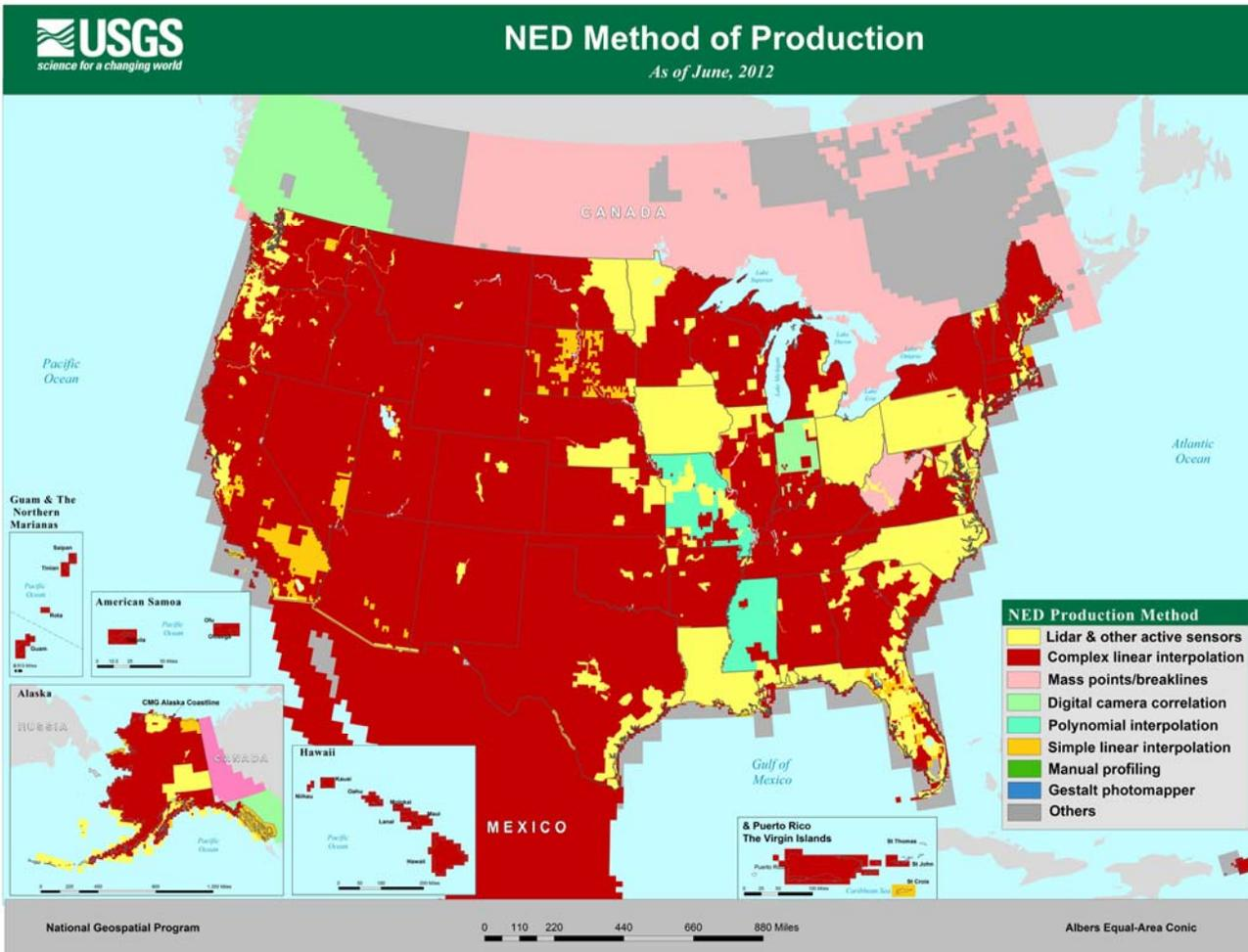
Figure 11. NED source data by production method – June, 2012 release.
