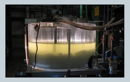
Why: Reduce risk of unexpected technical problems in supplying waste to the Waste Treatment Plant by testing systems that collect waste samples during feed and that mix different types of waste together to optimize chemical properties for incorporation into glass.
