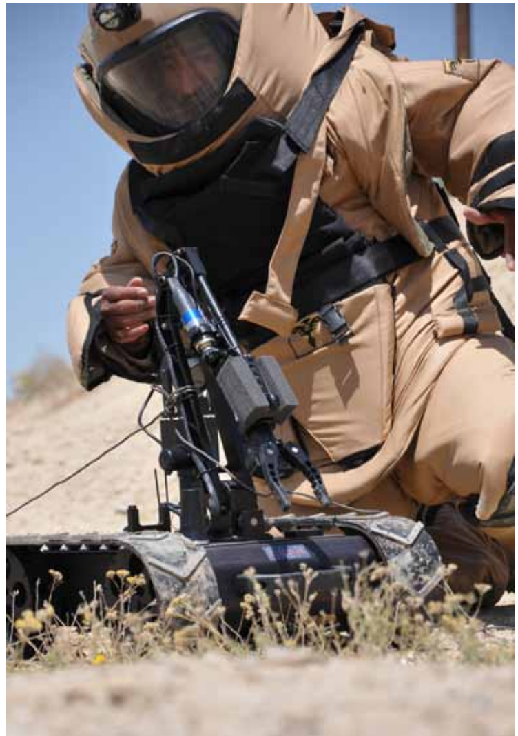
Afghan Army Explosive Ordnance Disposal Student Sgt. Zahidullah Khairkwa adjusts an MMP30 EOD robot while wearing a bomb suit during a training exercise at the Kabul Military Training Center. photo by Mass Communications Specialist 1st Class (SW/AW) Chris Fahey, NATO Training Mission – Afghanistan.
