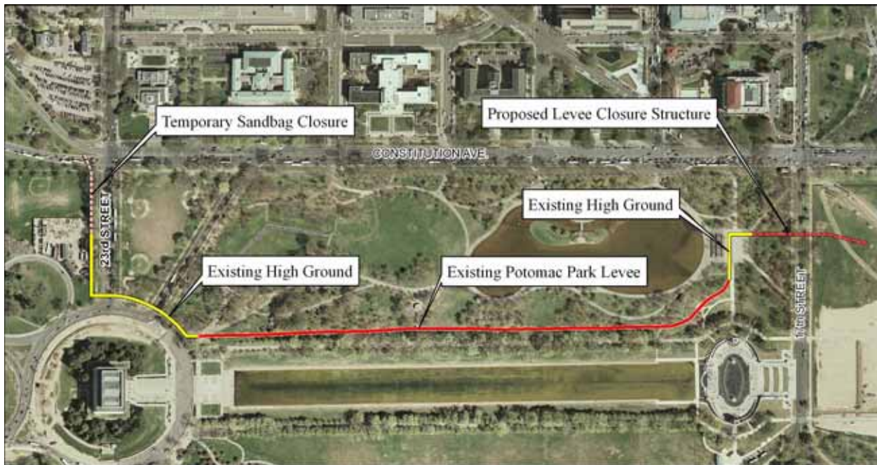
Figure 1. Potomac Park Flood Protection System
