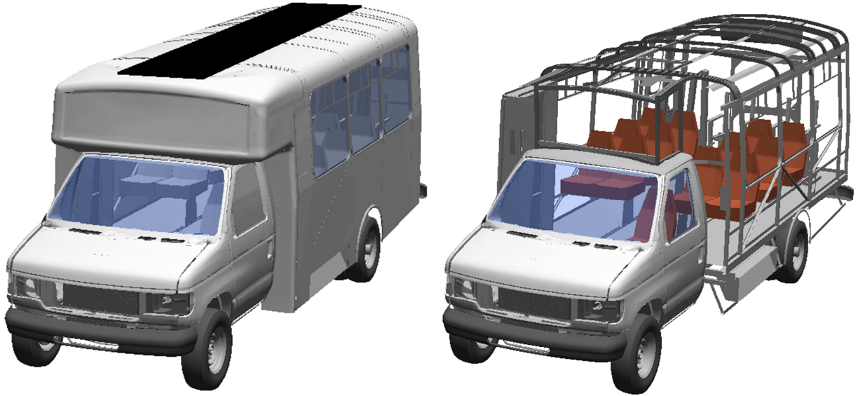
Figure 6.8: Residual space compromised by the bus structure. View of complete bus (a), view without skin (b)
