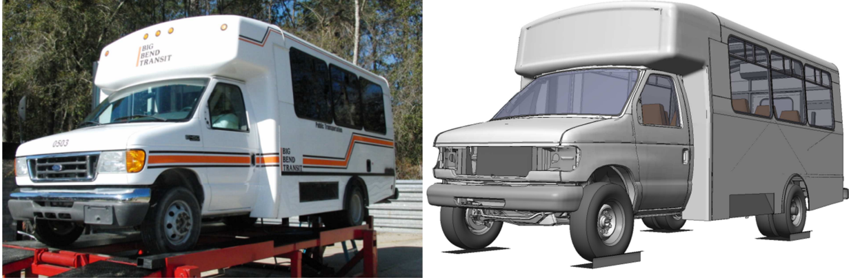
Figure 1.2: The bus selected for a rollover test (left) and its FE model (right)
