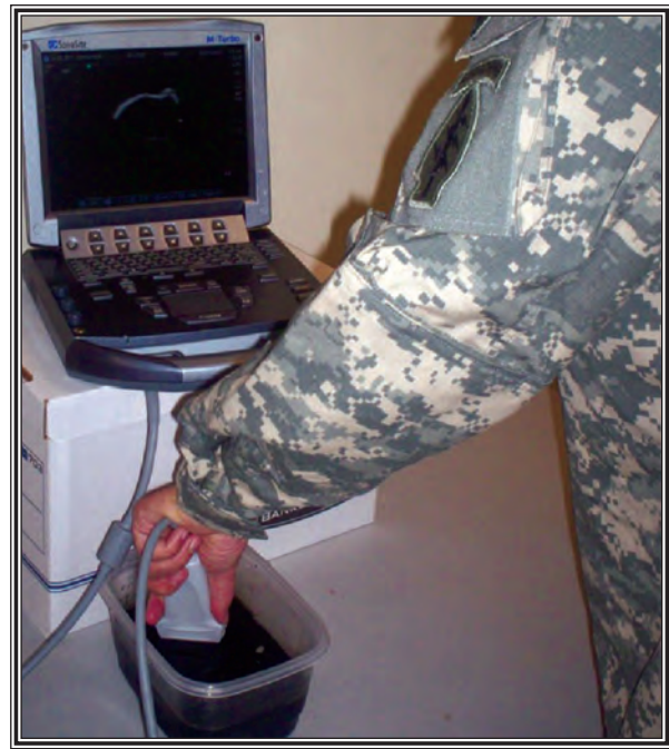
Figure 2: Fracture detection of the opaque study model via the SonoSite M-Turbo portable ultrasound.
