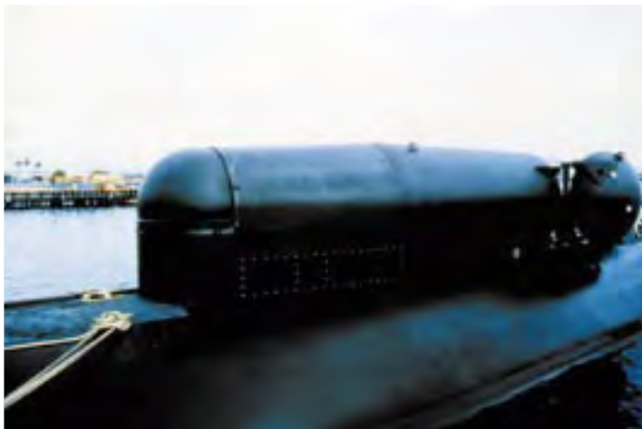
Dry Deck Shelter (DDS) for SEAL Delivery Vehicle (SDV) Photos courtesy of USN
