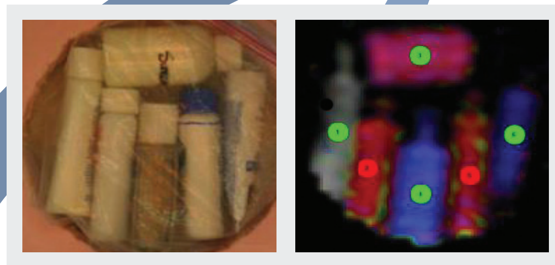
Hazardous materials may still be able to pass through airport security as long as they are contained in 3 oz. containers or smaller. MagViz and CoilViz are able to detect hazardous materials such as the 40% H 2 O 2 detected in bottles #2 and #5. Red light = bad liquid. Green light = OK liquid.
