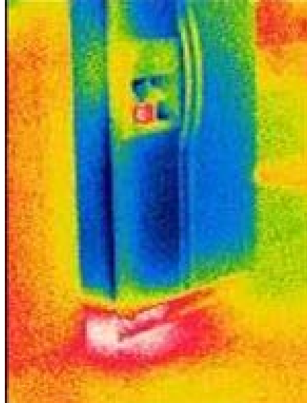
Figure 12. Infrared image of 25-ft 3 refrigerator showing heat rejection at the base of the unit, but also warm temperatures near through the wall ice and water access. The unit was using 4.4 kWh/day prior to replacement in January 2011.
