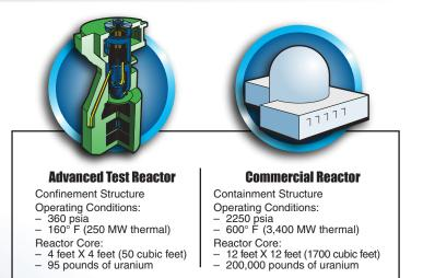
Key ATR parameters compared with those of a commercial pressurized water reactor.
