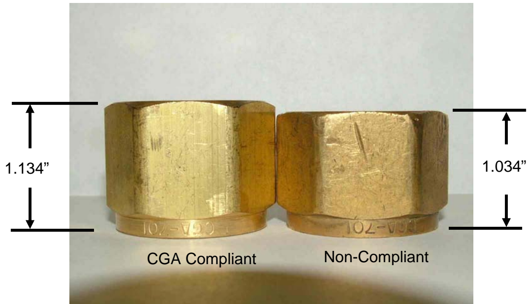
Measured length (shown upright) on non-compliant and CGA compliant high pressure fitting (nut)
