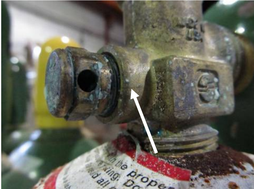
Figure 3 – View of cracked cylinder valve. Arrow points to crack.
