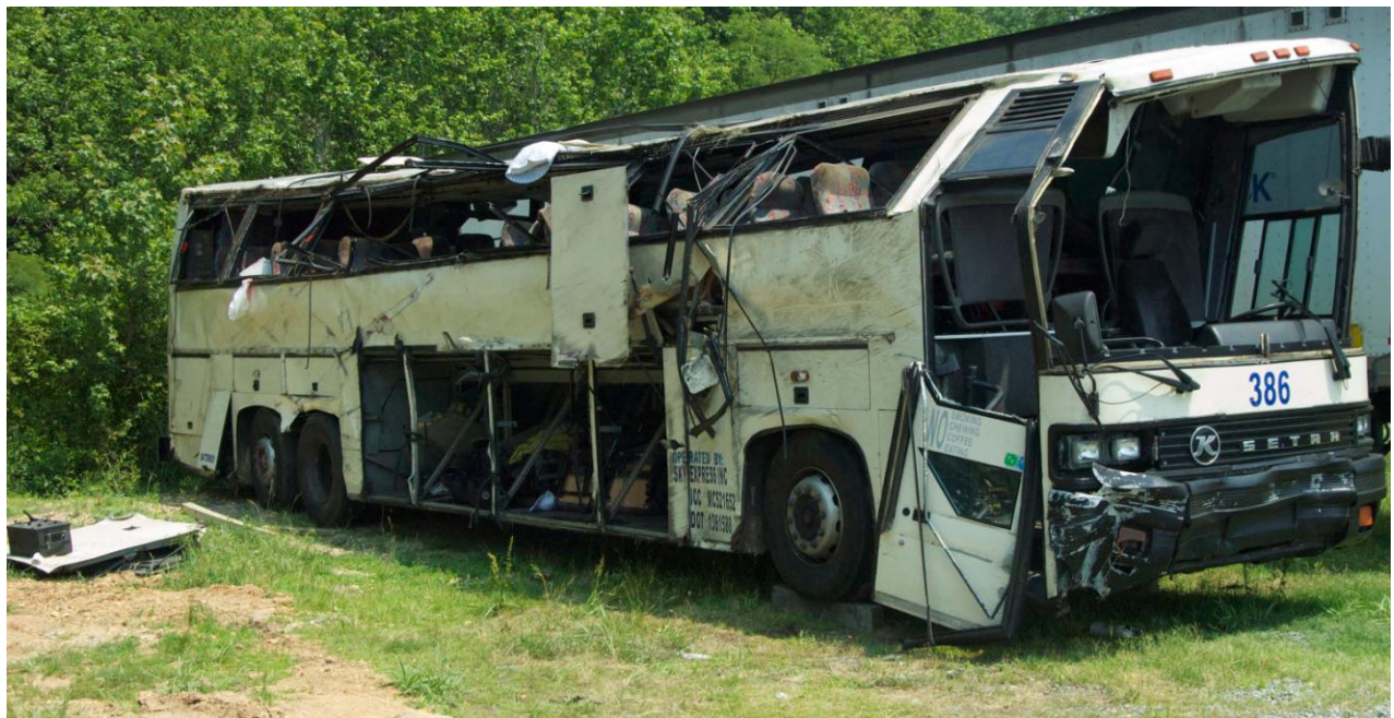
Figure 9. Damage to the passenger side of the motorcoach.
