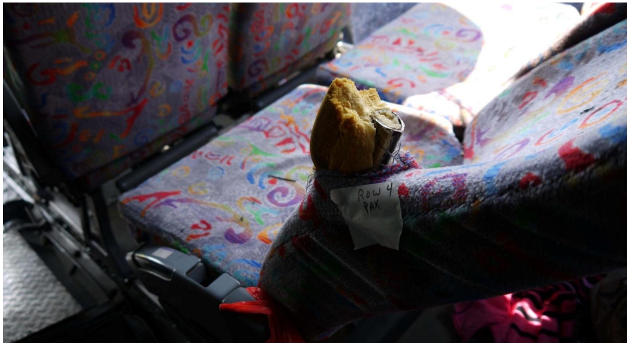
Figure 6. Damage to the aisle seat in row 4 on the passenger side of the motorcoach, showing that the collapse of the roof was so forceful it broke the seat structure.
