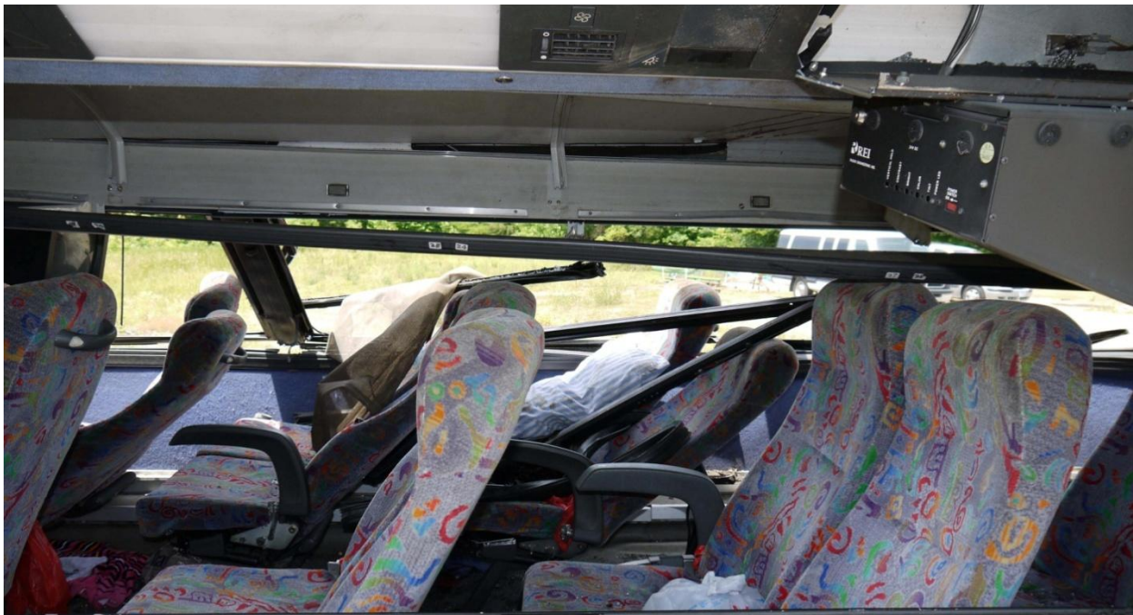
Figure 5. Passenger seats in rows 6 to 8 of the motorcoach after the vehicle was righted following the accident, showing the extent of the roof crush. (Note: The maximum roof crush, or roof deformation, was greater than seen here. It is common for a vehicle structure to “spring back” somewhat after an impact.)
